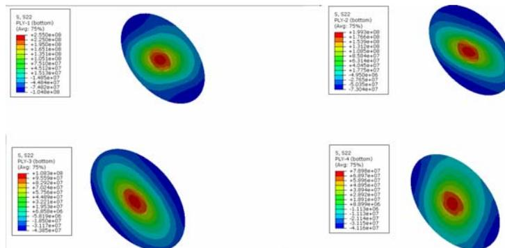
Looking at the input data table for strength values and computed stresses from damaged model in transverse direction in this data table and contours and comparing them it could be seen that a ply was failed.
