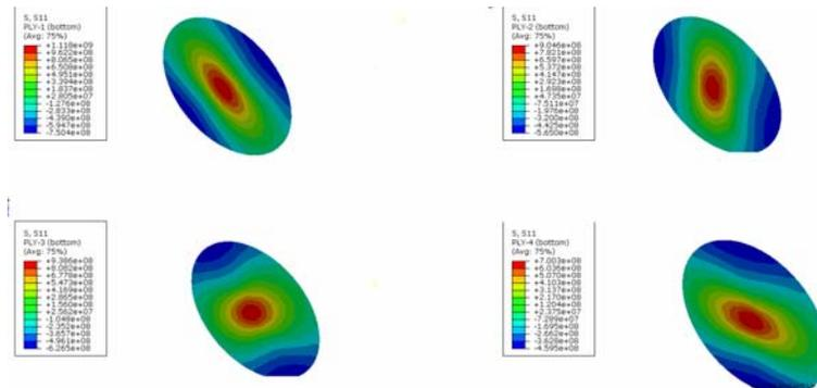
Looking at the input data table for strength values and un-damaged stresses in principal directions in this data table and contours and comparing them with the given strength values it could be seen that no ply was failed.
