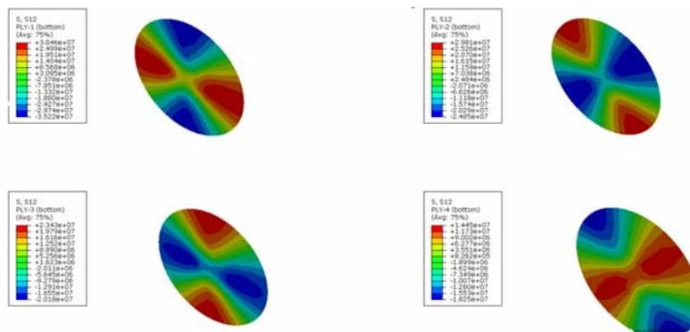
Looking at the input data table for strength values and un-damaged stresses in in-plane shear stresses in this data table and contours and comparing them it could be seen that no ply was failed. Using the given strength parameters and the computed stresses in the Tsai-Hill and Tsai-Wu criteria it was found that no ply fails.
