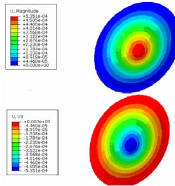
Magnitude and displacement values in the out-of-plane direction shown that there was a change in the values and values were bigger than the un-damaged model means that a ply was failed under the applied load (constant load).
