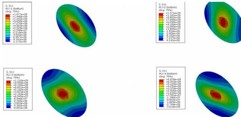
Looking at the input data table for strength values and computed stresses from damaged model in principal directions in this data table and contours and comparing them it could be seen that a ply was failed.
