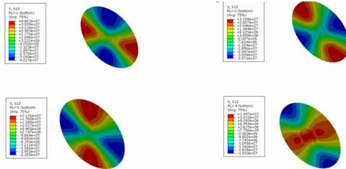
Looking at the input data table for strength values and computed stresses from damaged model in in-plane stresses in this data table and contours and comparing them it could be seen that a ply was failed. Using the given strength parameters and the computed stresses in the Tsai-Hill and Tsai-Wu criteria it was found that a ply fails.
