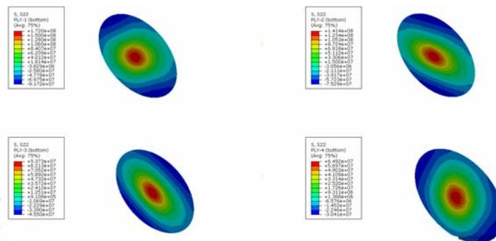
Looking at the input data table for strength values and un-damaged stresses in transverse directions in this data table and contours and comparing them it could be seen that no ply was failed.
