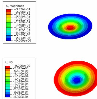
Magnitude and displacement values in the out-of-plane direction shown that there was no abrupt change in the values and values were reasonable means that no ply fails under the applied load (constant load).
