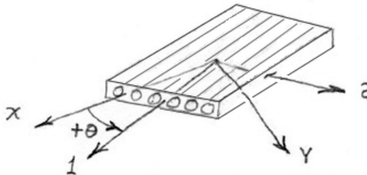
$$\begin{Bmatrix} \sigma_1 \\ \sigma_2 \\ \tau_{12} \end{Bmatrix} = \begin{bmatrix} Q_{11} & Q_{12} & 0 \\ Q_{12} & Q_{22} & 0 \\ 0 & 0 & 2Q_{66} \end{bmatrix} \begin{Bmatrix} \epsilon_1 \\ \epsilon_2 \\ \gamma_{12}/2 \end{Bmatrix} \tag{2-1}$$
